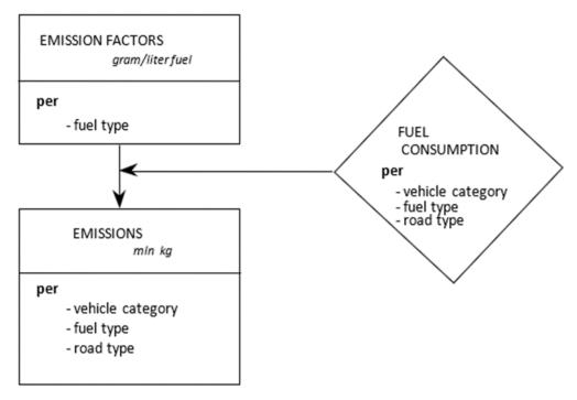
Figure 3.2 Methodology for calculating emissions of SO2 and heavy metals (cadmium, copper, chrome, nickel, zinc, lead, vanadium) due to combustion of motor fuels
