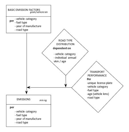
Figure 3.1 Methodology for calculating emissions of CO, VOC, NO<sub>x</sub>, N<sub>2</sub>O, NH<sub>3</sub>, and PM<sub>10</sub> due to combustion of motor fuels
