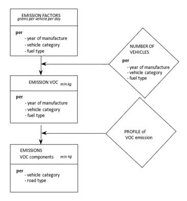
Figure 3.4 Methodology for calculating emissions of VOC components caused by evaporation of motor fuels
